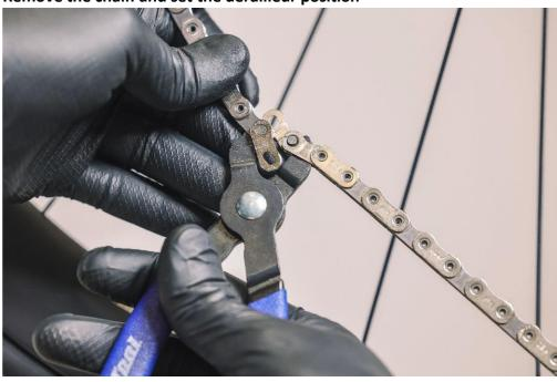
Using chain pliers, remove the quick link. IMPORTANT: Shift the derailleur into the highest position on the cassette (TOWARDS THE LARGEST COG OF THE CASSETTE)
