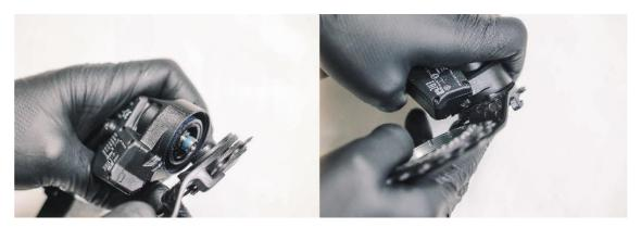
Without mounting the spring, match the D-shape of the clutch with the D-shape of the HOLLOWcage® then rotate the cage to the point where the cage's stopper is past the recess (stopper) on the derailleur. Memorise cage position and then remove it.
