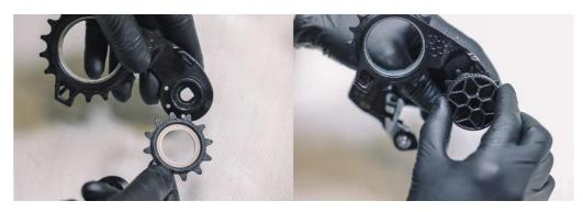
Mount the upper pulley wheel and tighten the lockring with the lockring tool to about 3-4Nm. To do that insert 8mm allen key to the lockring tool for final adjustment.
