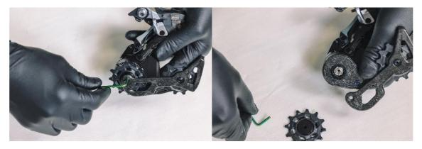
Using a 2.5 mm allen key to unscrew the bolt holding the upper pulley wheel. This will allow you to rotate the cage plate and gain access to the special locking nut holding the cage to the derailleur.
