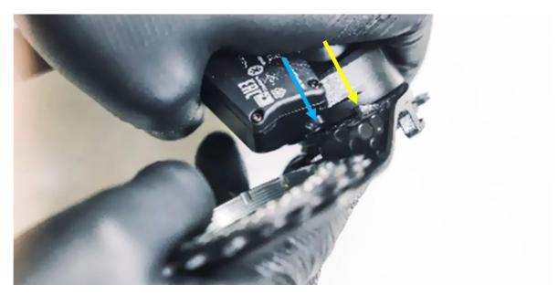
IMPORTANT: It is crucial to remember the position of the cage's stopper (yellow) in relation to the stopper on the derailleur body (marked with blue arrow).
