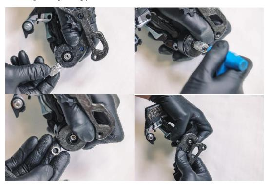
While holding the cage firmly, pressing it against the derailleur body, use provided tool and Torx T30 key to open and remove the locking nut holding the cage to the derailleur.
