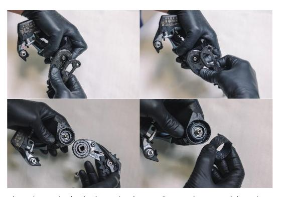
Release the spring tension by slowly rotating the cage. Remove the cage and the spring.
