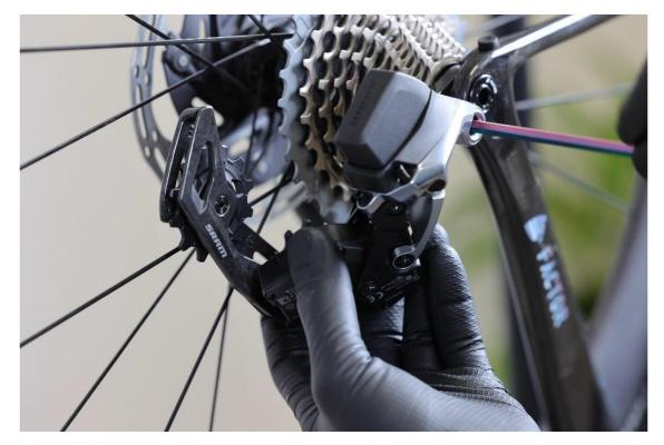
Using a 5 mm Allen key, unscrew the main mounting bolt an remove the derailleur
