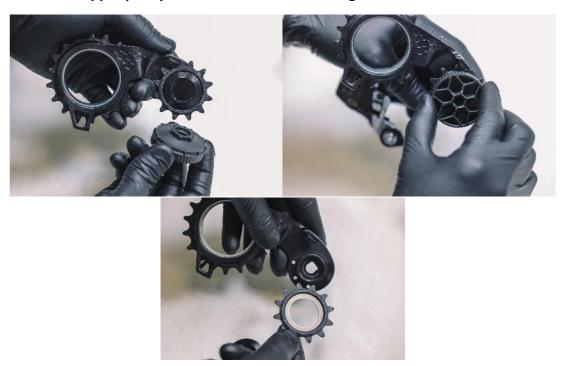
Use provided lockring tool to open the lockring holding upper pulley wheel.
